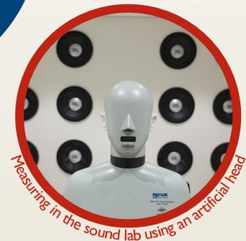
Measuring in the sound lab using an artificial head
